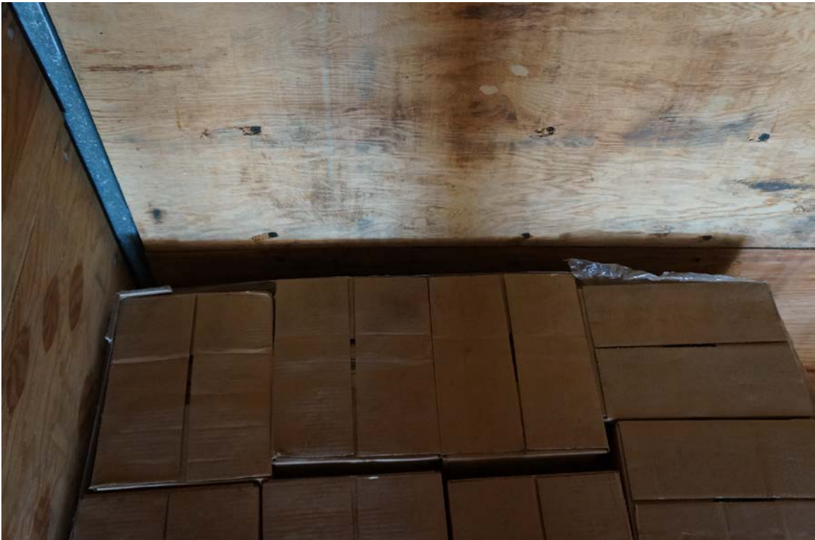
Longitudinal void space of 4 in. between the 1 st pallet and end wall on the left side after the reverse 6 mph impact.
