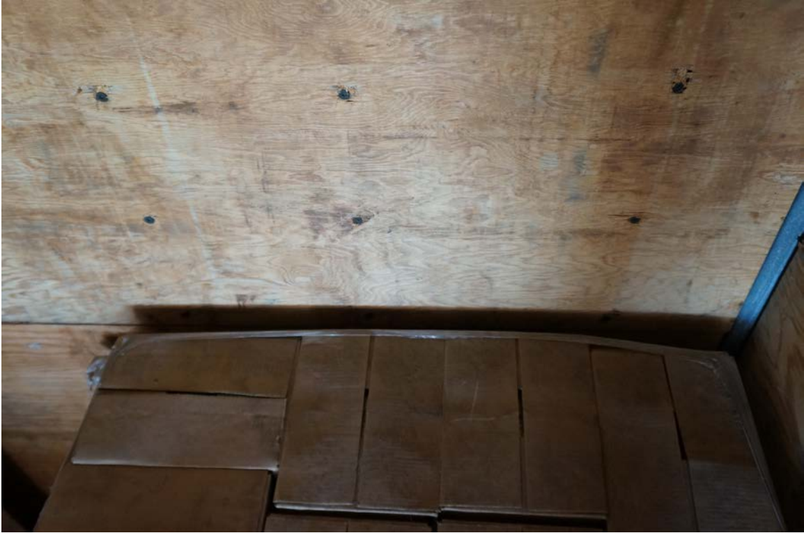
Longitudinal void space of 3 in. between the 1 st pallet and end wall on the right side after the reverse 6 mph impact.
