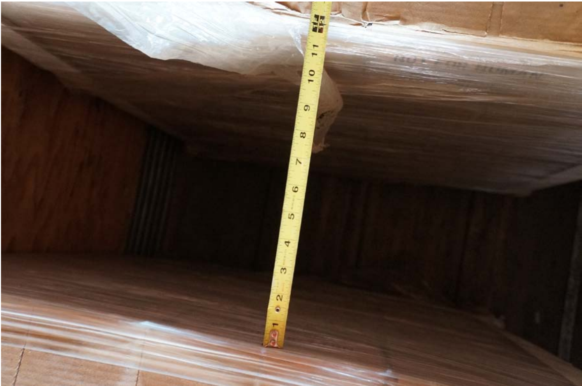
Longitudinal void space of 12 in. between pallets stack 3 and 4 created from the reverse 6 mph impact.
