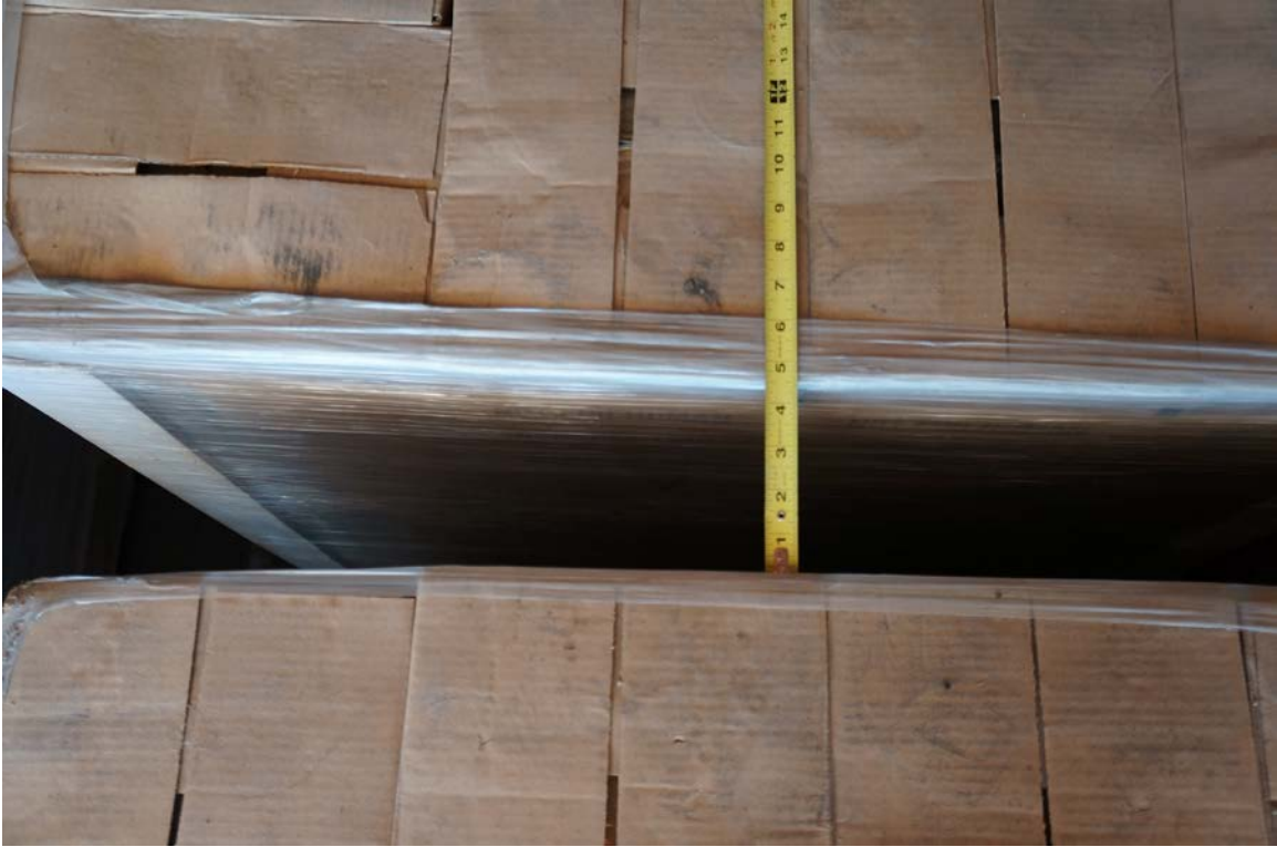
Longitudinal void space of 4 ½ in. between pallets stack 8 and 9 created from the reverse 6 mph impact.
